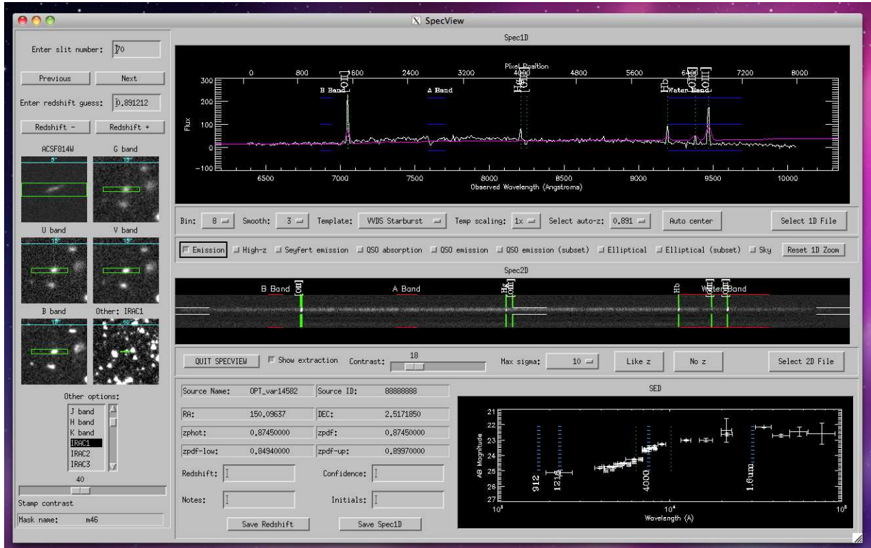
Fig. 2.— The SpecPro widget interface, small version. In this image, the “Show extraction” button has been selected, causing the slit to be overlaid on the stamp images.
